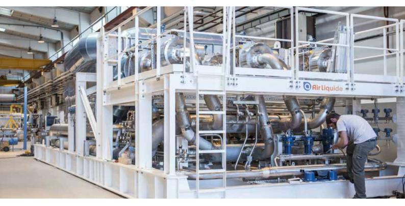
The Air Liquide Turbo-Brayton cooling system is an optimal solution for natural gas liquefaction. Combining performance, reliability and compactness, it can be used for liquefying biogas, natural gas or flare gas as well.
