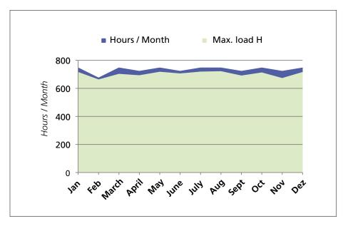
Typical electricity production of a biogas plant (h/month), The graph demonstratet that biogas plants are producing under full-load eletricity almost continuously.
